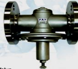
*Low Pressure Type Direct-Activated Pressure Reducing Valve (Stainless Steel 316) Pressure Adjusting Range : 0.2~1.5 kgf/cm 2 0.01~0.2 kgf/cm 2
