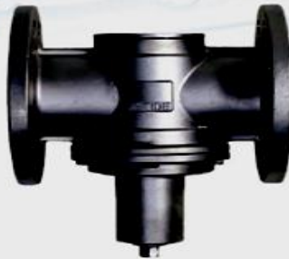
*Direct-Activated Pressure Reducing Valve (Cast Iron/Flange Type) Valve Body Testing Pressure : 21 kgf/cm 2 Maximum Applied Pressure: 16 kgf/cm 2
