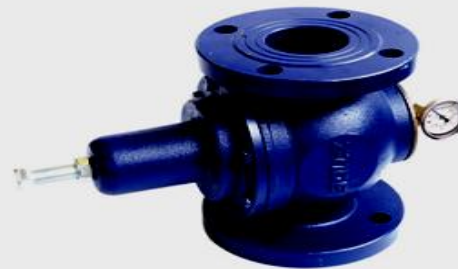
*Direct-Activated Pressure Reducing Valve (Cast Iron/Flange Type) Valve Body Testing Pressure : 21 kgf/cm 2 Maximum Applied Pressure: 16 kgf/cm 2
