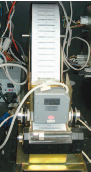
Each of these Class II machines contains a roll of tickets and a scanner which scans the bar code on each ticket.
