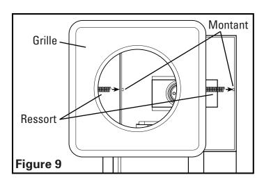
Install a 250 watt maximum, R-40 Type A heat lamp (not included) into the socket and center the grill around the lamp.
