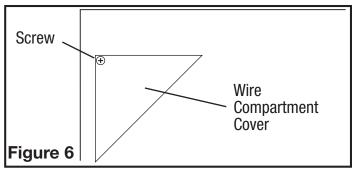
Internal Wire Compartment: Remove the screw holding the venturi in place. Lift the venturi up and at an angle to slide it out of the housing (Figure 7). Remove the wire compartment cover screw and place the cover in a secure place (Figure 8).
