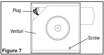
NOTE: If the fan motor plug is connected to the fan housing receptacle, unplug so the blower assembly can be completely removed.
