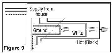
NOTE: The fan's receptacle wires might need to be pulled outside compartment for connection. Only pull the three loose wires outside of compartment. Additional wires will be present.
