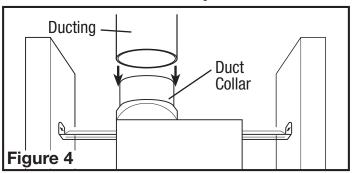
2. Ensure duct joints and exterior penetrations are sealed with caulk or other similar material to create an air-tight path to minimize building heat loss or gain and to reduce the potential for condensation. Place/wrap insulation around duct and/or fan in order to minimize possible condensation buildup within the duct, as well as building heat loss or gain (Figure 5).
