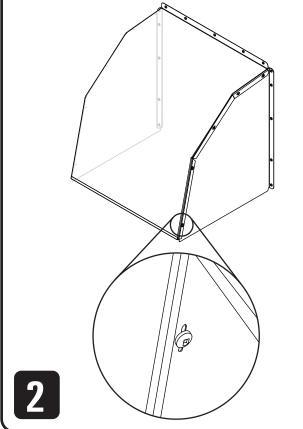
If mounting weather hood over a shutter or other inlet, ensure that hood placement will not block shutter movement.
