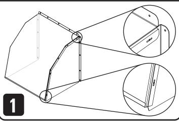
To secure assembled unit, join the edges and tabs together using the included #10 x 1" Square Head Tek Screws as shown below. (On sizes 12".30" use 5 screws for each side, on 36" use 10 screws per side, and on 48".50" use 11 screws per side.)
