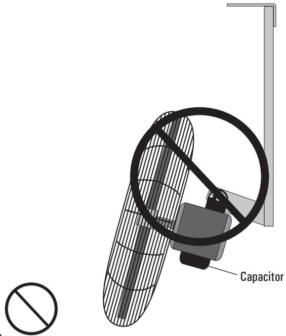
Do NOT mount bracket horizontally. The included bracket was not designed to be mounted this way and cannot withstand the structural stress caused by the weight and movement of the fan. Mounting the bracket and fan this way will void the warranty.
