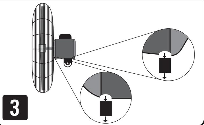
Attach fan to bracket. Insert bracket flag in between the motor flags and secure using the center holes on the motor flags with (1) 3/8" x 1-1/4 hex bolt, (2) 3/8" washers and (1) 3/8" nylock nut as shown in step 4a. Using the crescent openings on the motor flags, install the (1) 1/4" x 1- hex bolt, (2) 1/4" washers and (1) 1/4" nylock nut as shown in step 4b. Adjust the fan to the desired angle and tighten hardware to secure fan angle.
