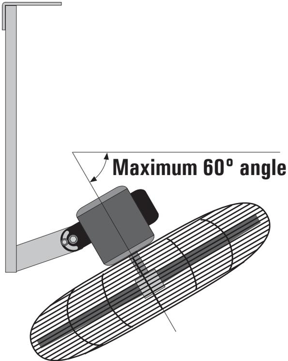
Do NOT mount fan with capacitor on the bottom. This can cause moisture to build up in the capacitor cap and short out the capacitor. Mounting the fan this way will void the warranty.
