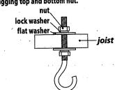
11/2" from installed J-hook mounting bolt, drill a small pilot hole for mounting the J-hook secondary bolt.
