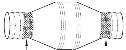
Use Nylon Ties or Sheet Metal Screws and Over-Wrap with Duct Tape
