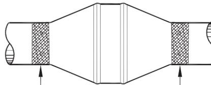
Use Sheet Metal Screws (1" Max) and Over-Wrap with Duct Tape
