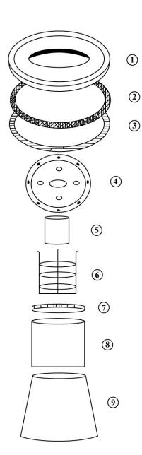
PART NO. QTY. REQ. **REFERENCE** DESCRIPTION 15 GAL. LID W/ MTG. PLATE & GASKET LID GASKET LID EDGING GASKET FLOAT MOUNTING PLATE **FLOAT** FLOAT CAGE **BAG CLAMP** FOAM FILTER BAG DACRON FILTER BAG
