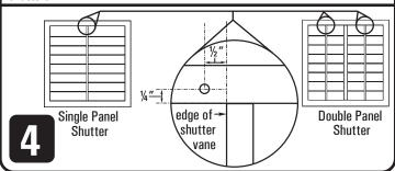
Hook one end of Return Spring into hole drilled in step 4. Hook the other end of the Return Spring around the rivet and spacer for the 3rd louvre from the top. For Double Panel shutter you will have to do this for each panel. See illustration.
