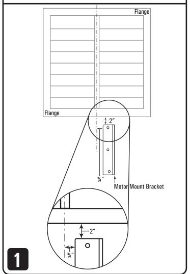
Secure the Motor to the Motor Mount Bracket using the 4 included Hex Head Flange Screws as shown.
