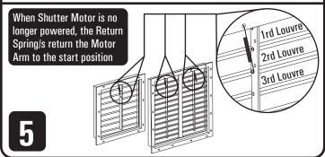
Insert an S-Hook into the first available hole below the Return Spring in each tie bar so as not to interfere with the movement of the Return Spring. Attach the end of the chain to the S-Hook in the tie bar.
