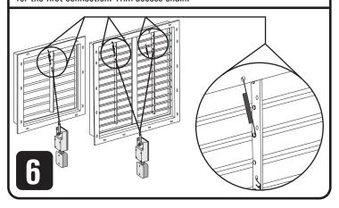
Supply power to the Shutter Motor. Watch the movement of the Shutter Motor and Shutter Panel. Ensure panels do not bind during opening or closing.
