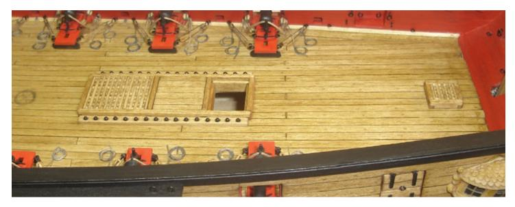
ing and glued into position. The smaller hatch on this assembly will be left open and the companionway will soon be built over it. See the photo showing the large coaming completed with the gratings and cover boards installed.
