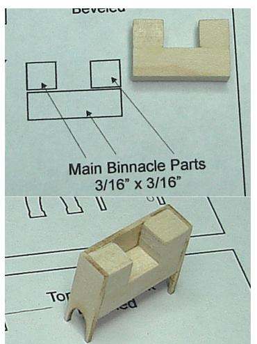
Before you glue the finished binnacle on deck it should be noted that it was secured to the deck with wooden battens. Glue a (1/32" x 1/32") strip to the inside edge of the binnacle's legs as shown on the plans and the final photo below.
