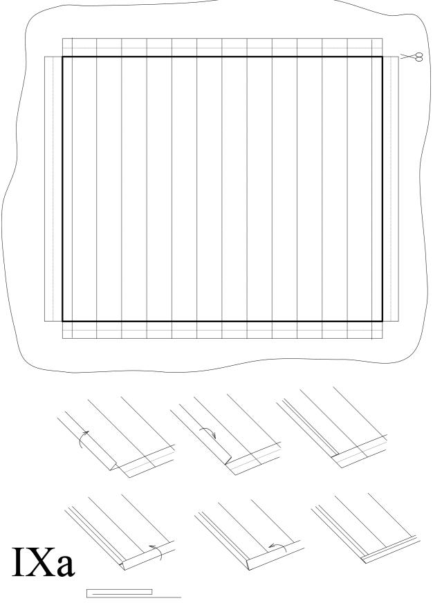
b) To the circumference of the sail sew on a rope 62 so that in the corner of the sail will eyes with diameters about 3mm. Then tie ropes 68 to sides of the sail.
