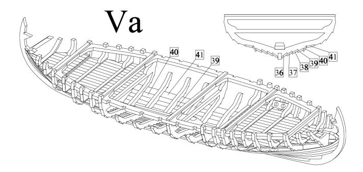
b) First glue frames 48-53 to the planks 41 and frame 27. Then bend beams 54 into needed shape and then glue them to the hull. Finally glue to the bow and stern parts 55 and 56.
