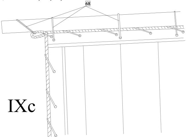
d) Tie the sail by ropes 68 to the hull and to the bar 69.
