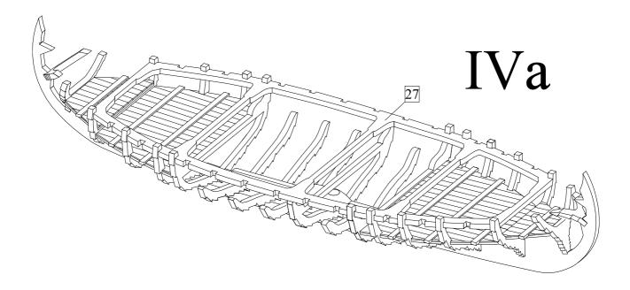
b) First glue transverse beams 28 to the frame 27. Then glue frames 29-35 to the transverse strips 26 and to the frame 27. Finally glue to the frames 14 a board with holes 75.
