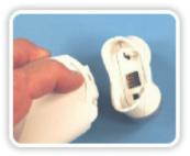
To reset the device, first remove the Trinity Facial Trainer (microcurrent) attachment by pressing the release button and lifting the attachment off.
