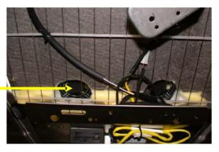
□ Place the fans towards the front of the cushion, forward of the seating area. This location is usually under the occupants thighs where the load is minimal. Recheck the location for obstruction of the seat pan and confirm that the load area will not be significant. If the fans are placed under the occupants seat area (Ischea bones), undue stress and possible air restriction will occur and will void the warranty.
