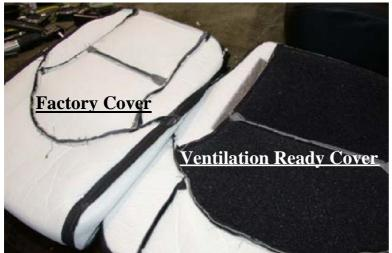
Photo shows factory cover on the left and new Ventilation Ready on the right. Black reticulated foam is sewn in to replace the factory foam backing.
