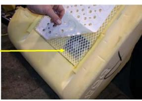
☐ Using a marker, trace the fan location.
