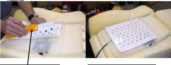
Peel the adhesive backing and apply to the spacer material
