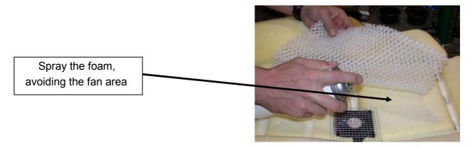
□ Lay the spacer material over the seat surface making sure that the material conforms to the foam
