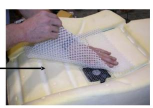
Position the heating element and peel the adhesive strip and apply over the spacer material
