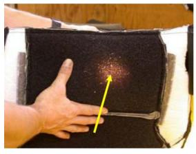
Photo shows perforated leather cover with reticulated foam sewn in. The cover is held up to a light showing the permeability of the cover
