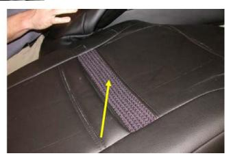
Photo shows a breathable panel sewn into the rear of the back cover allowing air to enter into the cover and to the fans. (recommended to increase performance but not required for system functionality)
