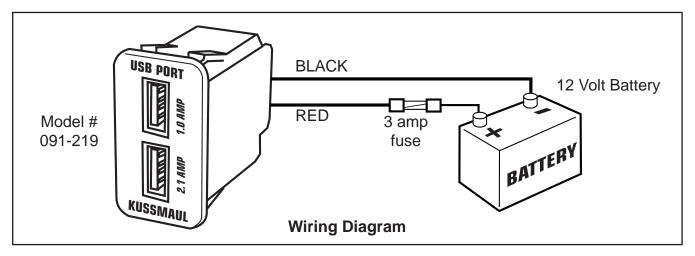
**Current Limit Protection -** The outputs of the USB charger are automatically current limited to approximately 3 Amps during overload and short-circuit conditions. During this condition, the LED will be extinguished. If an overload or fault condition is suspected, immediately disconnect all connected USB devices. The LED will illuminate and the outputs will return to normal operation as soon as the overload or fault condition is corrected.
