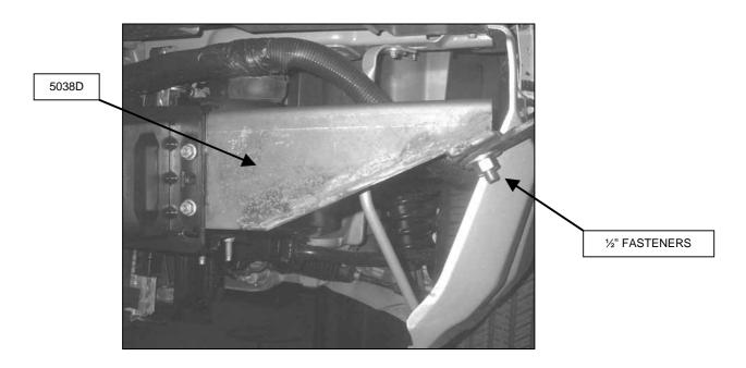
WARNING: It is the installer's responsibility, to tie wrap the wiring harness to the underside of the body to prevent the harness from coming in contact with the mounting bracket. Failure to do so may damage the harness and the vehicles electrical system.
