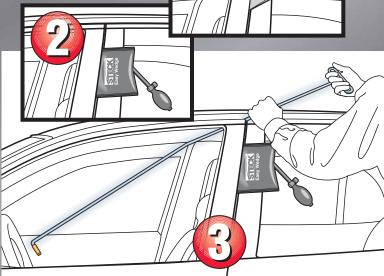
Actuate lock button, electric locks, or door handle with BigEasy to unlock.
