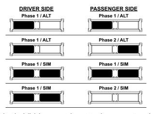
Synchronized lightbars, must be set to the same pattern. Not all patterns can be synchronized. Below are patterns available for SYNC.
