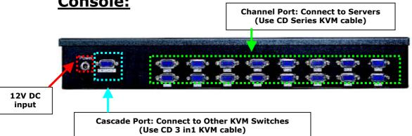
**12V DC input:** To connect to the external power adapter
