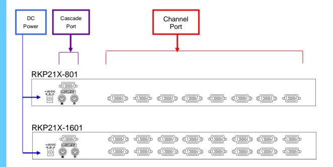
**DC Power** -connect to external 12V DC power adapter.
