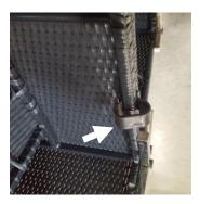
3. Push the clip and rotate it around the framework. The clip should not take much force to snap in place.
