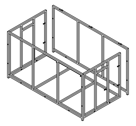
3. Attach the back piece to the partially assembled storage box. The back has part of the hinge assembly attached on the top side.
