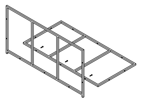
1. Take the front and bottom piece of the storage box and attach both pieces together using the provided screws and washers. Hand tighten all screws before fully tightening it for the full assembly.
