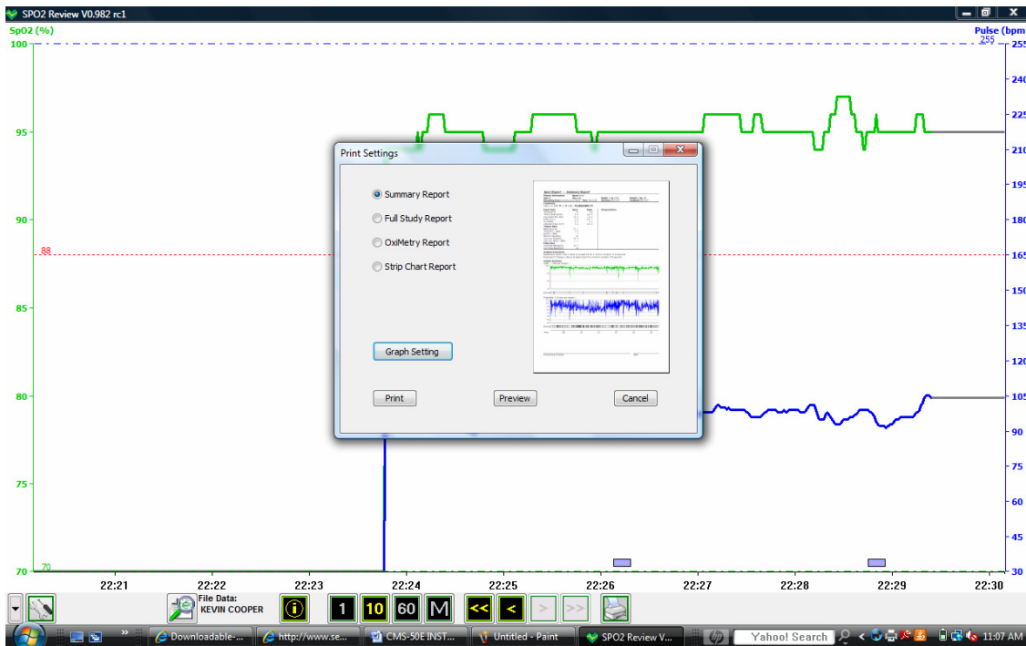
(Screenshot after hitting printer button. You will have the option of which report you want to print from Summary Report, Full Study Report, Oximetry Report, or Strip Chart Report).
