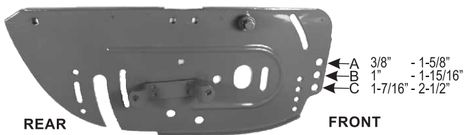
FIGURE 9: Use the front roller assembly cutting height adjustment holes and height adjustment lever to set the cutting height of the mower.
