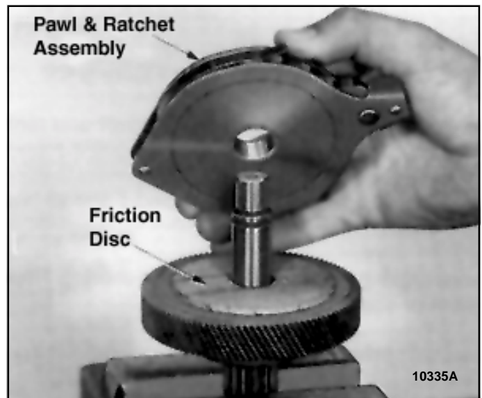
Figure 5-8. Removing Pawl and Ratchet Assembly From Load Brake Shaft
