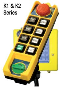
transmitters have 12 buttons for up to five motion control. Each comes also with E-Stop, Key Switch, and on/off. Each has 2 to 7 programmable auxiliary outputs, alarm output, A/B output, mainline output, and light output. Operating range is 330 feet (100 meters), or up to 1000 feet (300 meters) depending on the environment.
