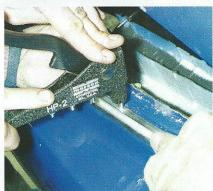
6 Once a snug fit is established, Terry drills rivet holes and temporarily rivets the trim using an aluminum rivet because steel is much harder to drill out. By the way, be sure to protect the paint.
