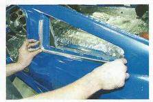
**5** Fit is challenging because no two Mustang bodies are identical. We're also working with extruded aluminum, which is rarely easy. Terry Simpson begins with a mock trim fit where the molding is fitted before permanent installation. Both bottom and top pieces are checked for fit at this time.
