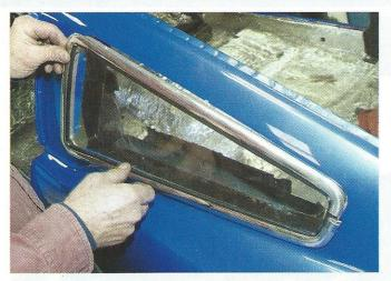
14 The window assembly is carefully fitted in place to where all rivet holes line up. This sounds easy, but it isn't. This is a very tight fit requiring exceptional caution. Terry is using 3M rope caulk between the molding and body to keep water and dust out.
