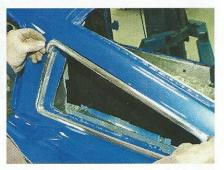
The upper half of the trim is test fitted to determine where it must be trimmed for proper fit.
