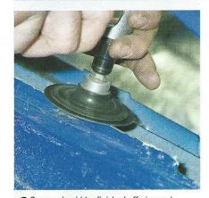
3 Seams should be finished off nice and smooth with a coat of primer to prevent corrosion. Had we known we were installing Shelby quarter windows, we would have done this during the bodywork before paint.
