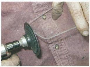
**9** Not only does extruded aluminum trim need to be massaged, so does the Plexiglas window. Because this window is made of soft plastic, it scratches easily. It's a good idea to leave the protective covering intact during installation.
