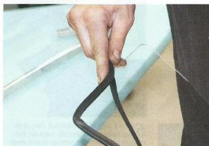
10 Window seal is installed using WD-40 as a lubricant. Because WD-40 evaporates, it makes a good temporary lubricant. Expect the molding fit around the Plexiglas to be tight.
