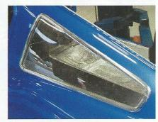
19 This is the way your finished Shelby quarter window should look. Extruded aluminum moldings are flush with the sail panel and Plexiglas isn't warped or wavy.
