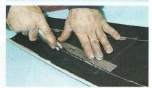
12 The panel is marked with masking tape and trimmed with a razor blade. Be careful and keep trimming minimal at first. You can always cut more, but you can never get back what you've cut.
