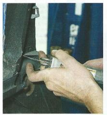
4 Interior body structure also needs to be trimmed as shown to make way for trim pieces.
