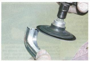
OThe molding is carefully trimmed to allow just enough gap between the upper and lower halves. You want at least an .060-inch gap to allow for expansion in the hot sun. If you don't trim for sufficient gap, the aluminum trim will expand in the heat and could buckle.
