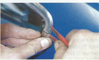
16 Molding end caps are carefully popped into place. It is easy to damage paint, so caution is crucial.
