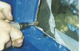
2 The fastback air extractor webbing must be cut out to make way for Shelby quarter windows. It is important not to cut out too much and compromise body structure integrity. Keep the sandwiched and spot-welded seams, which means don't go too far.
