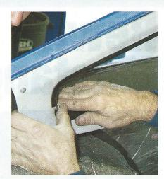
18 Inside fiberglass trim is installed next, with Terry first determining where the rivet holes will be. You can also use stainless steel trim screws. Before the inside trim goes on, paint the areas just inside the window flat black to hide imperfections. Ideally, interior trim will fit flush with the Plexiglas.
