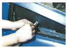
1 1 We're going with cool interior trim panels from Mustangs Plus. This means special trimming required just like you would with a factory trim panel. Begin with a straight edge from the window frame to the trim panel and mark accordingly.
