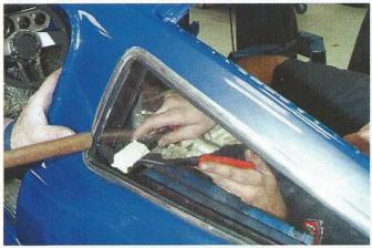
15 Terry leans hard on the molding to get the proper rivet hole alignment while Richard installs steel pop rivets inside. Richard places cloth between the rivet gun and Plexiglas to prevent damage.
