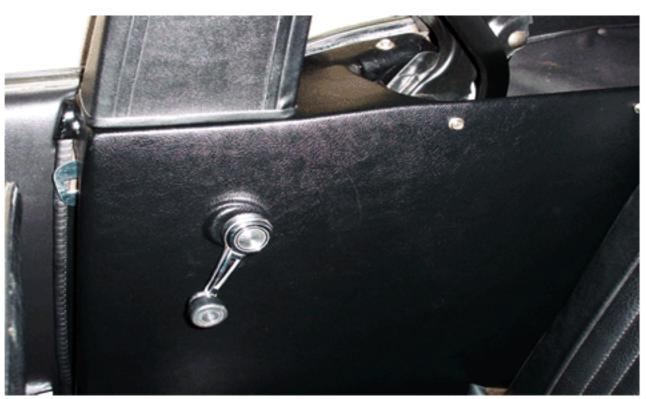
STEP 7: Install Shelby Side Panels (Install the Shelby side panels, with interior screws in various locations and reinstall window crank handle.)
