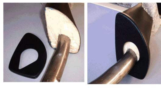
STEP 4: Glue bottom caps (gaskets) onto the roll bar.
