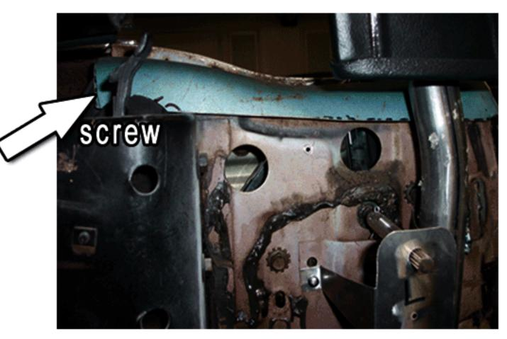
STEP 6: Install cut top section of stock trim panel. (Using the factory interior trim panel top from step1 install onto car using 2 screws one on top towards front and rear on inner side as marked in photo with arrows.)
