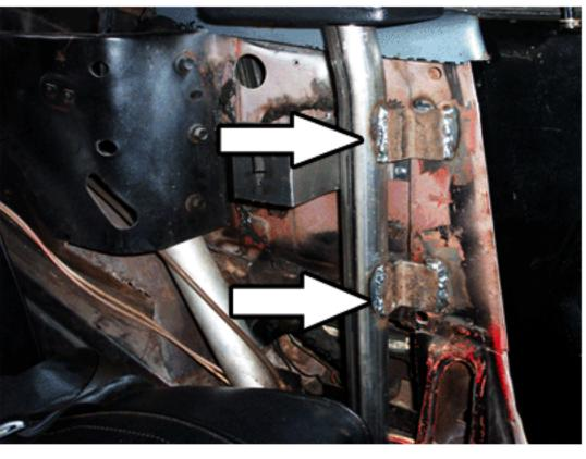
STEP 5: Test fit bar and tack weld in place (Check for top clearance and side panel fit, then measure and tack weld bar in place using supplied "L" brackets and the diagram shown. After fit is confirmed proceed to make your final welds as shown.
