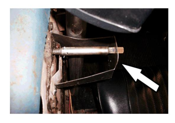
STEP 3: Install window crank shaft extensions and brackets. (Crank shaft extension is installed first using a cotter pin to attach it to the existing crank then the bracket is used to secure it in place, repeat for both sides of car)
