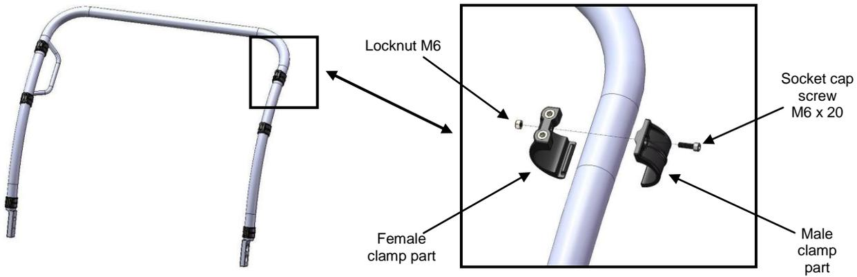
d) Install windshield to clamps using M6 x 16 knobs as shown. Adjust height position and level of the windshield to ensure good fit with hood. Once clamp positions are adjusted, tighten all screws with specified torque indicated below. **Over-tightening clamps to roll cage could cause parts failures.**
