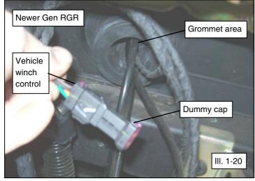
29. Connect the white harness connector to the winch contactor connector as shown. Access is gained by reaching thru the front bumper and thru the front gearcase access window to reach white contactor connector. Use cable ties (item #2) to secure the harnesses. (See illustration 1-8).
