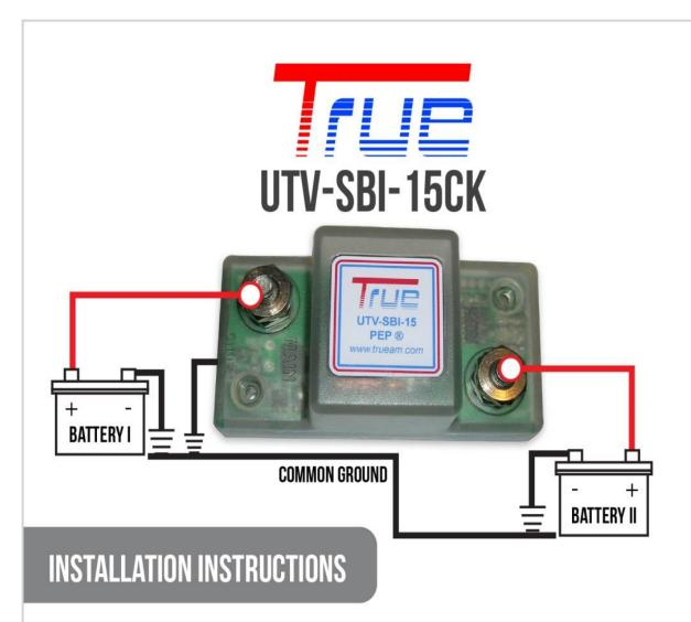
FYI: The SBI is designed ambidextrous so it cannot be installed backwards. Either stud can be connected to either battery's positive terminal.
