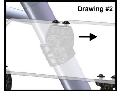
3. Pull gently on the windshield as per drawing #2 towards the front of the vehicle for the upper pivot to slide to the end onto the upper pivot cylinder adaptor.
