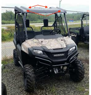
5. Install 2 spacer Blocks between rollbar and roof, 2 ¼"-20x2.5" bolts with ¼" USS washers on top side of roof through 3<sup>rd</sup> and 4<sup>th</sup> holes, 1.5" emt clamp around rollbar and secure with ¼"-20 nylocks
