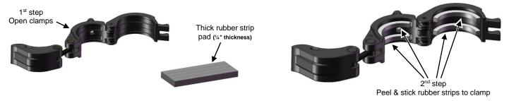
c) Attach the clamps to the roll-cage as shown below and pre-adjust tightening tension of all clamps. NOTE: Keep all clamp handles open as shown in step 3 below; this will allow you to move the clamps up or down when installing the windshield for the first time.
