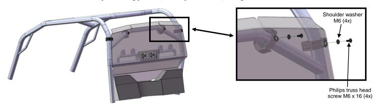
f) Using a ¼" drill bit, make 6 holes to the black panel located behind the seats using the windshield mounting holes as guide. Secure the lower windshield section using supplied push type retainers.
