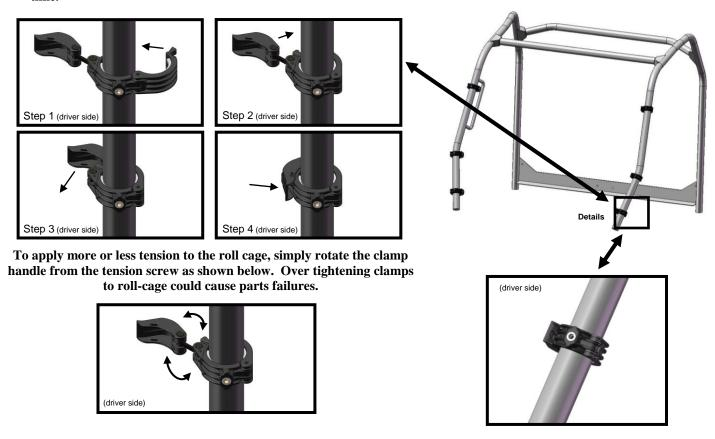
d) Install windshield to all clamps by using supplied hardware (Item F) without applying final torque. Adjust position of the windshield and tighten all knobs and all clamps to the roll cage. Ensure that the windshield is perfectly level before tightening. If the windshield isn't level, windshield functions will be affected. Over tightening clamps to roll cage could cause parts failures.
