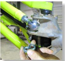
Secure tie rod bolt with a 10mm washer and 10mm lock nut.
