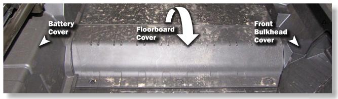
Remove the battery cover, front bulkhead cover, and floorboard cover from the cab to access the brake lines.
