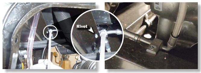
Remove the rivet and disconnect the front T-block from the frame (above the front differential). You may need to use an angle grinder to remove this rivet.
