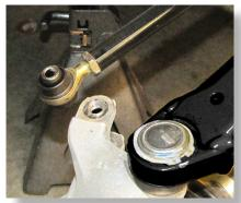
Disconnect the **tie rod** from the knuckle. **(15mm)**
