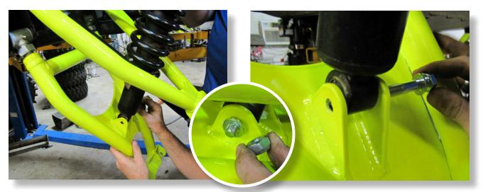
Install the shock to the lower arm shock tab.
