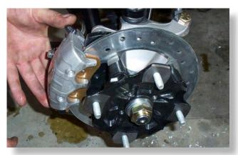
Connect the caliper to the hub assembly.
