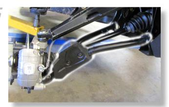
**Remove the Lower Arm FIRST** by removing the bolts at the knuckle (15mm) and the frame. **KEEP ALL FACTORY HARDWARE.**
