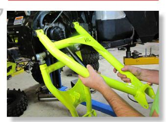
Connect the new upper arm (134U) at the frame using the factory hardware.
