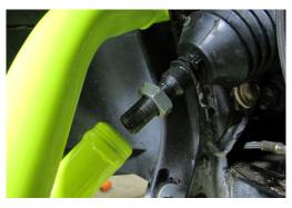
You will need to turn the steering wheel closer to the center to allow play in the boot. Slide the boot back down and secure it with an 11" zip tie.
