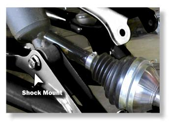
Disconnect the lower arm FIRST by detaching the arm at the frame, then disconnect the lower shock and sway-bar. KEEP FACTORY HARDWARE; it will be used to reconnect the new control arms.
