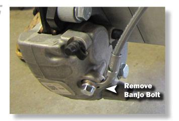
Disconnect the **stock brake line from the caliper**, if you have not done so already.
