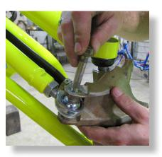
Run the 10X75 bolt through the tie rod.
