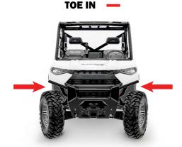
If the FRONT OF THE WHEELS are facing IN, adjust the tie rods IN or REDUCE the length of the tie rod.
