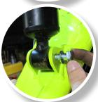
Use a 10X55 bolt followed by a 10mm washer to secure the UPPER shock to the lift bracket. Secure bolt with 10mm washer and 10mm lock nut.
