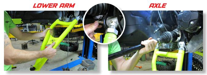
Install the new **lower control arm** to the frame, using the factory hardware.
