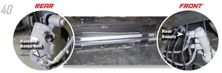
Disconnect the rear brake lines from the calipers. Have a container ready to collect fluid. Disconnect the rear supply line from the cylinder then remove it and the factory **REAR brake lines. It is faster to cut the lines since they will not be reused, but is not necessary.**
