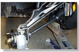
Disconnect the **Upper arm** by removing the **bolts** at the knuckle, sway bar, shock, and the frame. **KEEP ALL FACTORY HARDWARE**.
