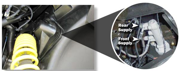
Remove the panel from the fender well on the (DR) side to access the master cylinder.
