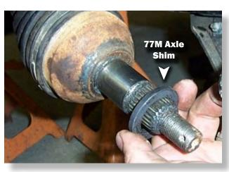
THIS STEP IS FOR 2018 MODELS ONLY. Install the (77M) Axle shim over the axle shaft. (TAPPERED SIDE GOES IN TOWARD THE AXLE)
