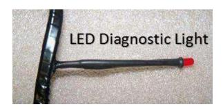
If there is a malfunction with an electronic part, the system will create a code to identify the problem. Each fault code is displayed by a series of flashes with through the fault light.
