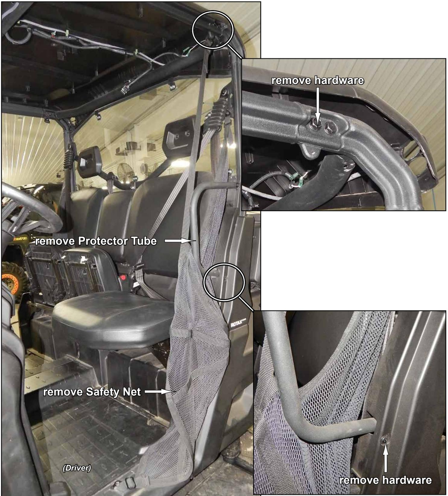
**Driver Door Installation:** do not tighten hardware completely unless noted.
