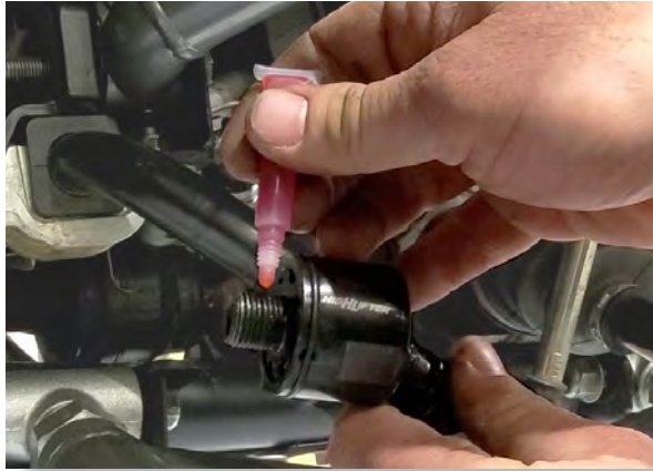
Use Red Loctite on threads of heavy duty inner tie rod.
