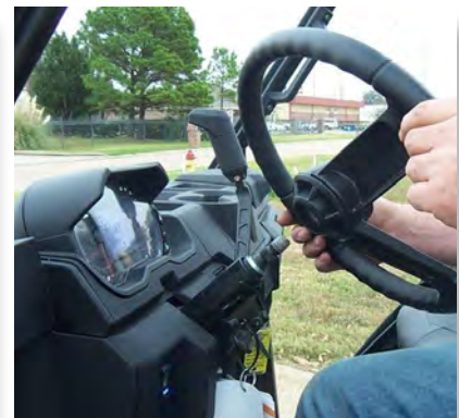
(C) Using a ratchet, turn the steering nut counter clockwise or left. Continue this until the steering wheel locks at full turn, then loosen the nut. DO NOT remove the nut yet.
