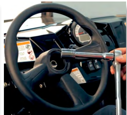
(C) Using a ratchet, turn the steering nut counter clockwise or left. Continue this until the steering wheel locks at full turn, then loosen the nut. DO NOT remove the nut yet.
