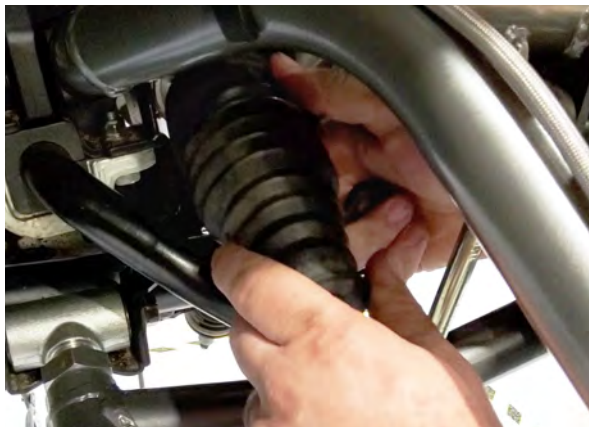
Install stock boot. Zip tie to boot to rack.
