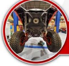
PLACE JACK UNDER THE CENTER OF REAR AND LIFT UNTIL THE WHEELS ARE OFF THE GROUND. BE CAREFUL TO SECURE PROPERLY SO IT IS STABLE ON THE JACK OR JACK STANDS. REMOVE THE REAR WHEELS.
