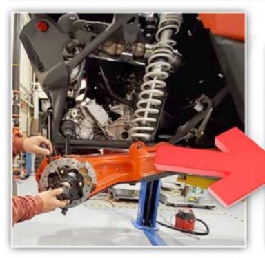
BEFORE YOU REMOVE THE BOLT THAT SECURES THE RADIUS BAR TO THE HUB ASSEMBLY YOU WILL NEED TO REMOVE THE BOLT THAT CONNECTS THE CALIPER TO THE HUB OR IT WILL HIT.
