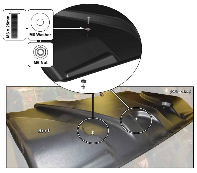
Align Roof to machine and tighten hardware completely
