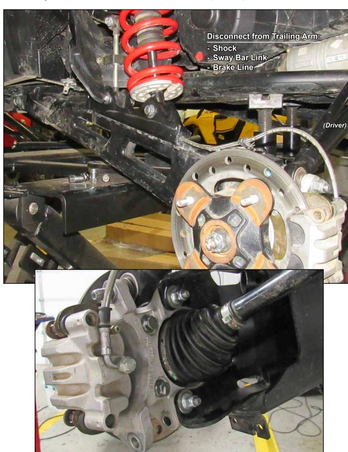
disconnect Lower RSL and remove Caliper
