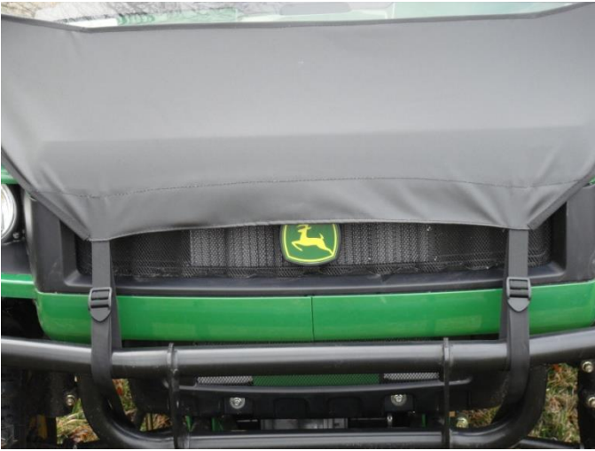
Figure 7.1 - attach Front Hood Straps to the vehicle front bumper – Do Not Fully Tighten Straps at This Time
