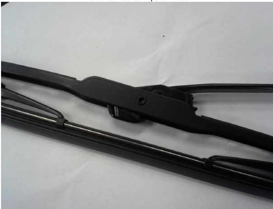
View onto installed wiper arm hook.
