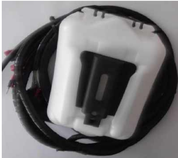
Harness and washer tank
