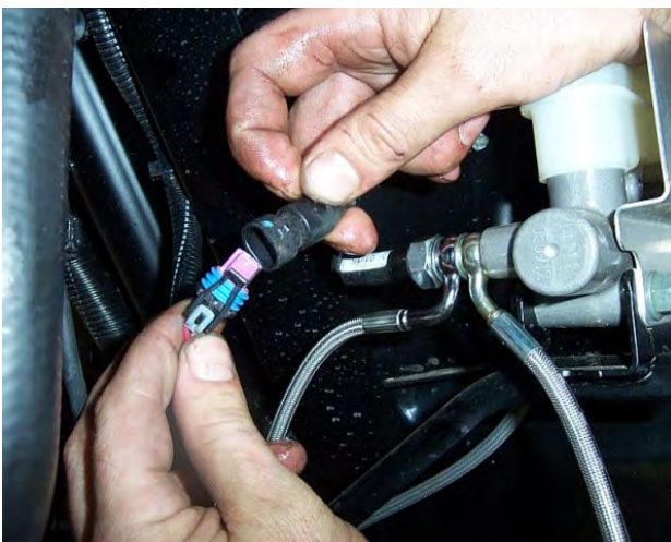
Use the right factory brake line that you removed to replace the left factory brake line. The left factory line will not be long enough once the new control arms are installed. Then connect all the lines back to the master cylinder using the factory hardware.
