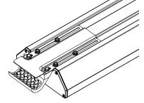
When the bolts are loosened, the bracket can slide to accommodate a variety of roll cages whose inside roll bar dimension is between 32.25" and 38.75" for the MUDSYS31, 43.0" and 49.0" for the MUDSYS41, and 49.25" and 56.0" for the MUDSYS46. Once the proper width has been established, these bolts should be retightened to a torque specification of 40-45 inch/lbs.
