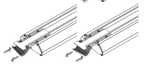
Each C-bracket has two (2) total bolts. These bolts can be loosened to adjust the clamp angle allowing it to mount to a variety of roll cages including those that are angled.
