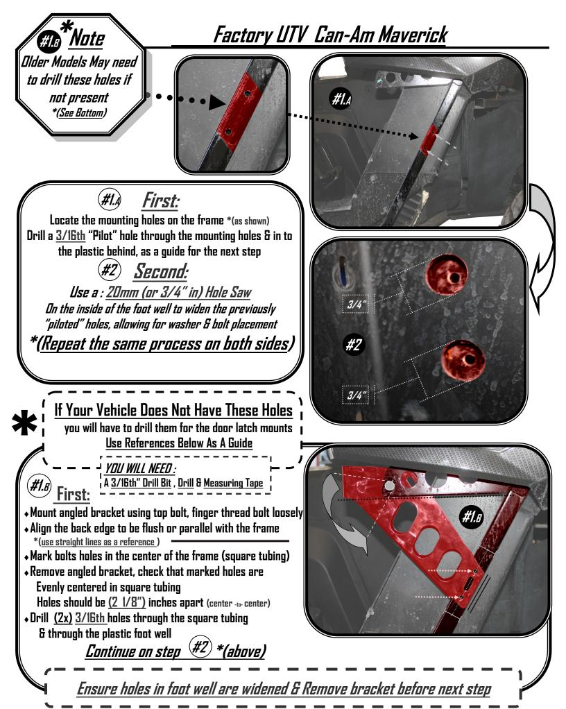
Mounting Instructions<br/>are the same on both sides4 seater models will install similarly<br/>with center hinge mount & latch.Cut & trim plastic as needed
