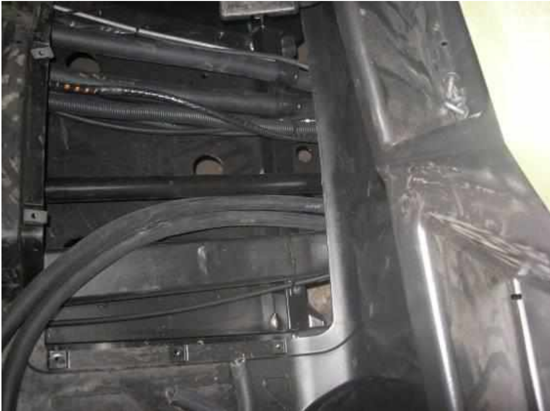
Water hoses in the floor tunnel.
