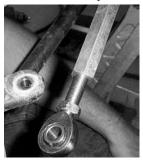
13. Using a  $\frac{1}{2}$ " drill bit or equivalent, open the hole of the knuckle assemble to  $\frac{1}{2}$ ".
