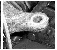
14. Take the ½ x 3" Hex Bolt and insert one of the Hi-Alignment spacers onto the bolt. Slide the bolt into the heim joint, then place another Hi-Alignment spacer onto the bolt.
