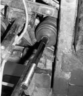
10. If you have not done so already install the jam nut back onto the rod end. Then, place the hex bar onto the rod.
