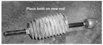
9. Connect the new rod to the rack and pinion and lid the boot over the joint. s
