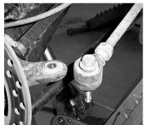
4. Cut the plastic boot bands from the boot on the rack and pinion. The boot end to the inside is going to be difficult to cut and replace.
