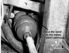
5. Once you have cut the bands pull the boot down to expose the end.
