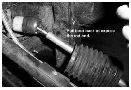
6. Using a wrench disconnect the rod from the rack and pinion.
