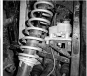
3. Disconnect the rod from the knuckle assembly.
