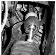
7. Now that you have removed the rod from the rack and pinion remove, end that connects to the knuckle assembly. Remove boot from the rod.
