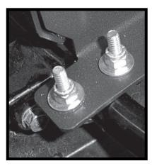
Connect the radiator to the rack using the  $\frac{1}{4}$  x 1" bolts, U-bolts,  $\frac{1}{4}$ " washers and  $\frac{1}{4}$ " lock nuts provided in the kit.
