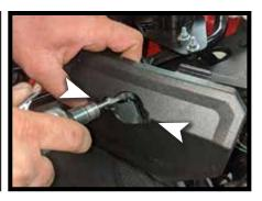
Locate the access panel and cut a 1 %" in hole in the center. If you DO NOT have a rotary tool we recommend you to use a 1/2 drill bit to drill out holes on the side for extra wiring space BEFORE drilling the 1 % hole.
