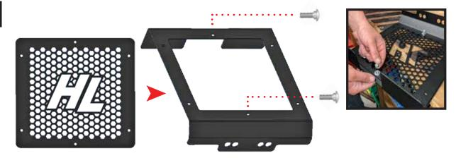
Start preassembling the the radiator mount by placing the face plate BEHIND the plate frame and install the two 1/4 X 3/4 carriage bolts to the center bolt holes then back it with the two 1/4 washers and 1/4 lock nuts provided.
