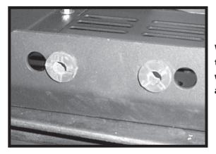
Where the bottom of the stock radiator attaches to the frame there are two **rubber grommets** that you will need to **remove** and place in the two center holes at the base of the new **face plate**.
