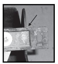
You will need to trim the stock radiator fan brackets, so that it will fit into the new shroud.
