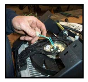
Cut the blue and green wire half way between the plug and the motor on the back of the fan.
