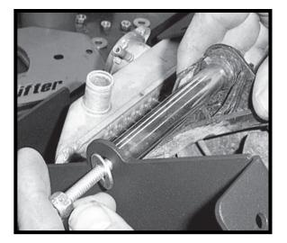
Next use the two large spacers and 1/4 X 5 bolts to connect the fan to the brackets.
