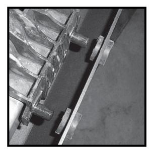
Once they are installed you will need to then insert the bottom of the radiator into the grommets.
