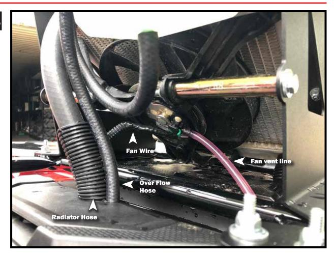
IMPORTANT: Place the remaining loom around the hose to keep it from rubbing on the rack and plastic fenders. If the hose is left unprotected the vibration of the hose against the rack and fenders will form a hole, causing fluid to leak out, potentially RESULTING IN ENGINE DAMAGE.
