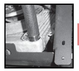
**Connect 2ft of hose** to the bottom of the radiator. Secure the hose to the lower portion of the radiator with the **clamp** provided.
